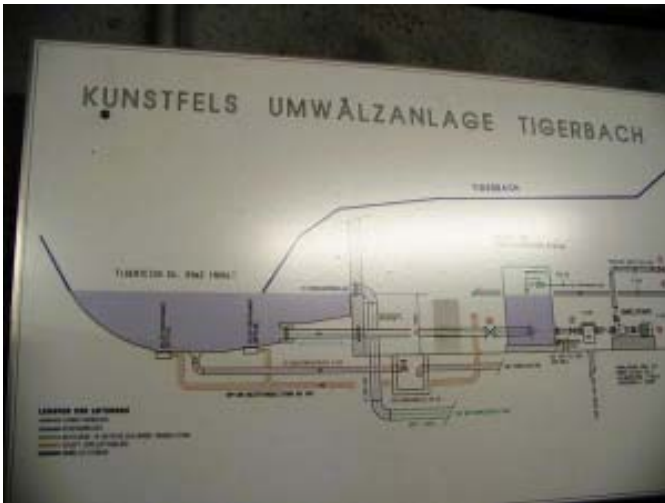
Water Recycling - The water of the tiger pool is filtered and circulates through an artificial creek. ©Monika Fiby, 2004
